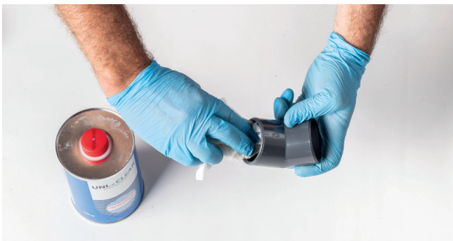
Using a clean paper towel soaked in cleaner primer remove traces of dirt or grease from the outer surface of the pipe and from the internal surface of the socket of the fitting leaving the surfaces softened
