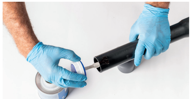
Apply a normal layer of adhesive and cover the pipe axially
