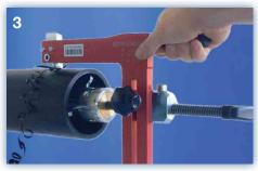
3. Peel the pipe up to the mark in order to remove the oxidation layer. Use a rotational peeling tool. Do not use sandpaper, metal files, etc.
