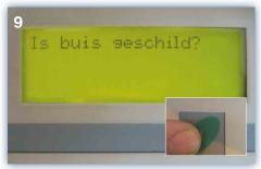
9. Press Start (green button). The control box will ask if the pipe has been peeled. If yes, press the Start button again, the control box will start welding.
