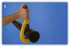
1. Check the PE pipe for damage, scratches and ovality. Ensure pipe ends are cut square and burrs are removed. Remove dirt.
