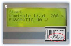
8. Check the jointing time on the fitting with the jointing time shown on the display. **If they do not match, do not start the welding process.**
