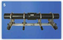
5. Remove fitting from the plastic bag. Slide fitting into pipe until it reaches the center stops of the fitting. Check the depth of the marking. If the fitting cannot be correctly inserted on the pipe due to ovality, the pipe will need to be re-rounded. Secure the pipe with pipe clamps.
