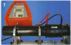
7. Connect the red fusion cable to the red pin and the black cable to the other pin by pulling the black sleeves of the welding plug backwards. Place the welding plug on the pins and release the sleeve.
