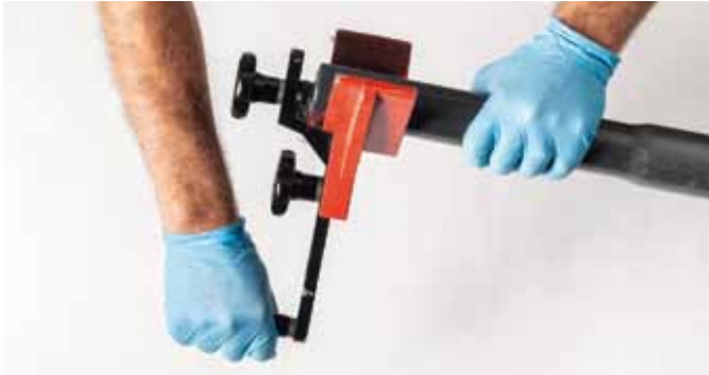
Cut pipes at right angles using a pipe cutter Chamfer pipe ends with chamfering tool or file
